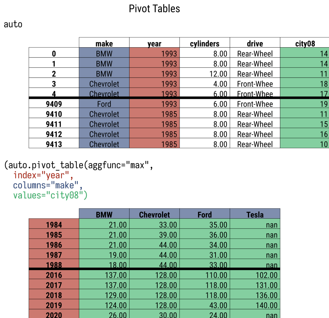
Figure 27.1: The .pivot_table method allows you to pick column(s) for the index, column(s) for the column, and column(s) to aggregate. (If you specify multiple columns to aggregate, you will get hierarchical columns.)
